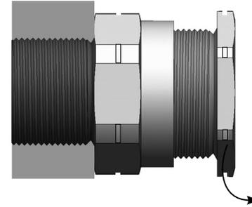
4. Only using finger pressure, tighten the seal nut until light resistance to tightening is met.
